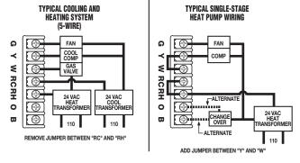
NOTE If you have an electric system and the blower does not operate after installation, find the electric/gas heat jumper on the back of the body. Move the jumper to the ELEC position.
